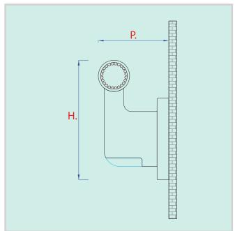
**DESCRIZIONE**Tubular handrail with main extruded continuos aluminum, diameter 40 mm.
