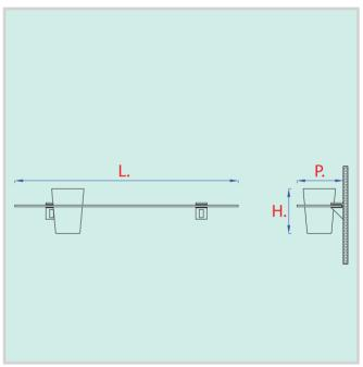
**DESCRIPTION** Straight support made of Polymers, including extractable glass.
