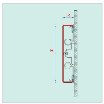
**DESCRIPTION** Shock-absorbing buffer height 200 mm.
